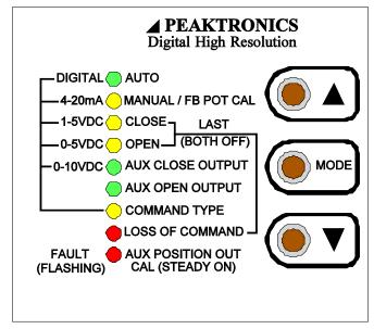
Figure 1 - Control Panel DHC-100x/200x Gen 1 DHC-300x
